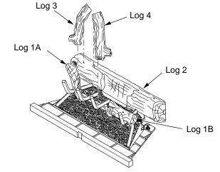
Figure 30 - Installing Logs 3 and 4
